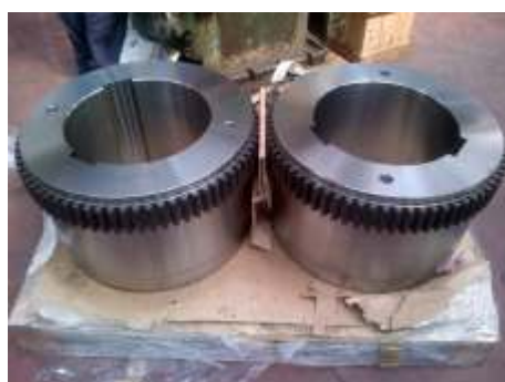
HEAVY DUTY GEAR HUBS WITH INDUCTION TEMPERING
