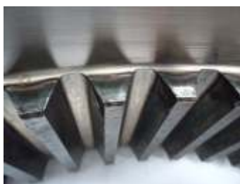
SLEEVE TEETH WITH INDUCTION TEMPERING
