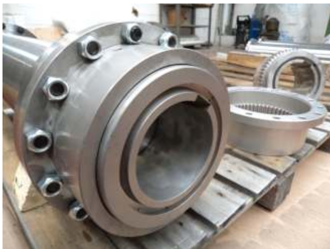
GEAR COUPLING WITH CONTINUOUS OIL LUBRICATION
