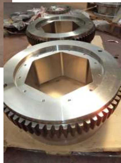
HEAVY DUTY GEAR HUBS WITH HEXAGONAL BORE AND TEETH WITH INDUCTION TEMPERING
