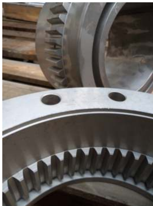
GEAR HUBS AND SLEEVES IN 42CrMo4 GAS NITRIDED
