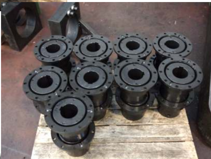
HALF GEAR COUPLINGS PROVIDED WITH HEAT TREATMENT: BLACK TREATMENT (NITRO - OXIDATION)
