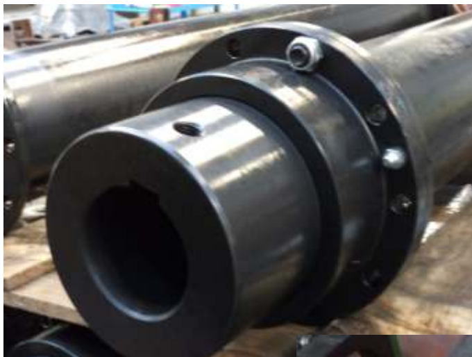
HALF GEAR COUPLINGS PROVIDED WITH HEAT TREATMENT: BLACK TREATMENT (NITRO - OXIDATION)
