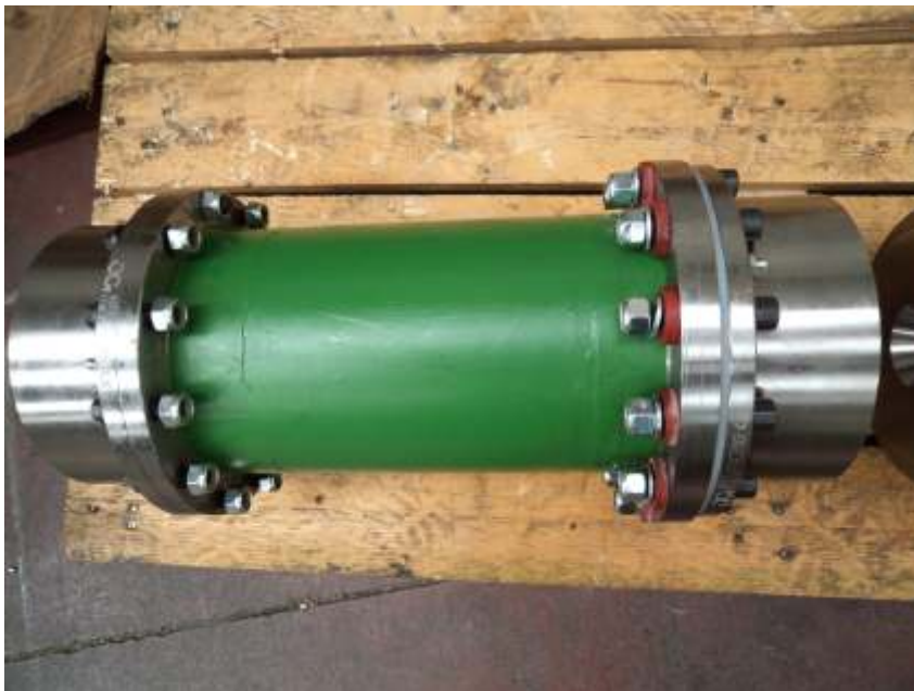
GEAR COUPLING WITH ELECTRICAL INSULATION AND TUBULAR SPACER
